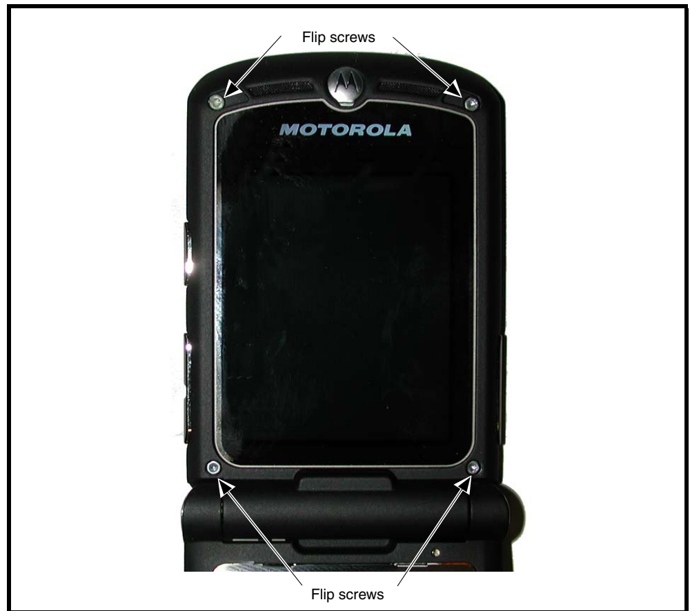
Figure 11. Removing the Flip Assembly Screws
