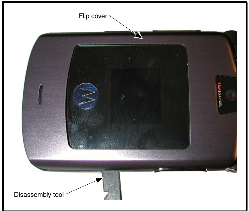
Figure 12. Separating the Flip Assembly Cover
