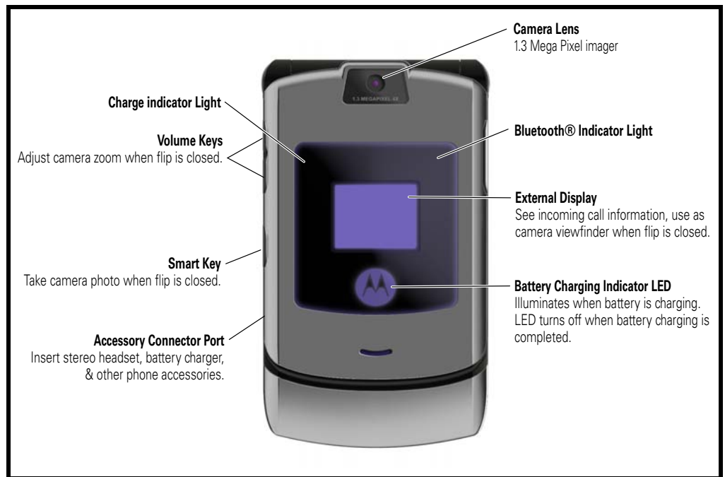
Figure 2. External Display, Keys, indicators, and I/O
